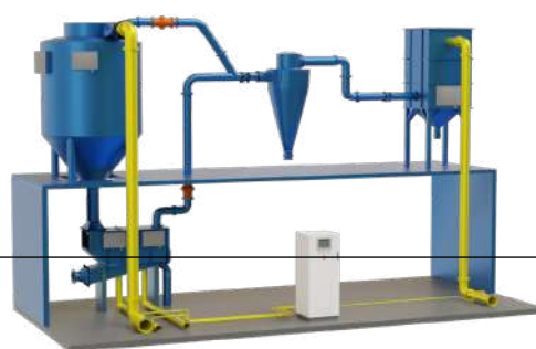
Figure 4. Hóbré CO monitoring system on a spray dryer.
