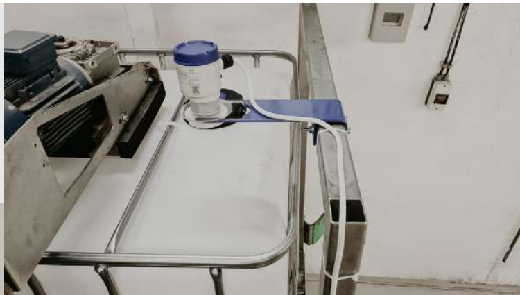
The IBC fill level is detected non-invasively from the outside
