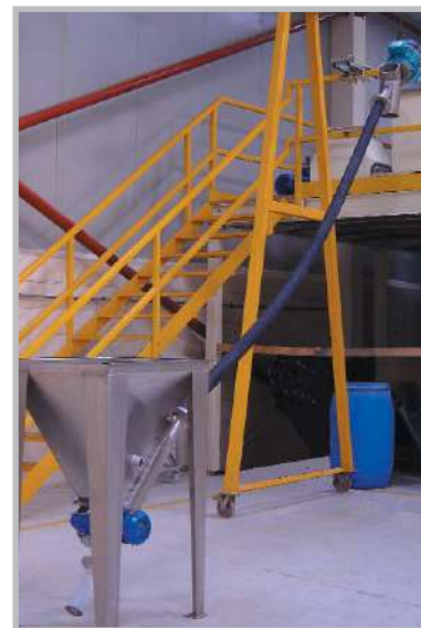
Our range of RHINOVEYOR Flexible Screw Conveyors are for very abrasive materials such as sand, cement and aggregates.
