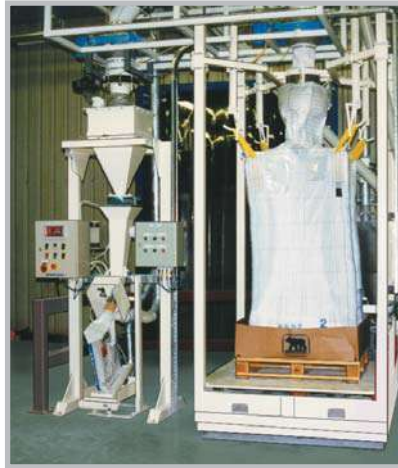
Filling system for bulk bags and 25kg sacks.
