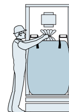
8. Bulk bag spout removed from filling nozzle and tied.
