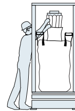
3. Liner or bag spout is attached to inflatable neck seal.
