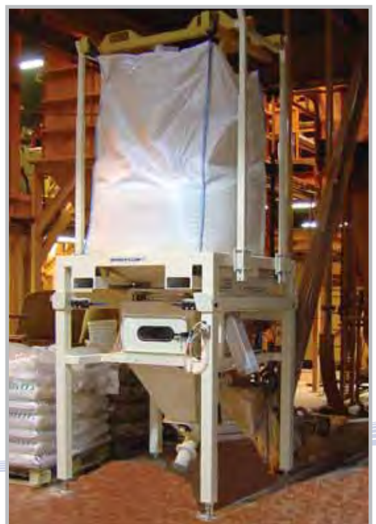
5. Bag loaded ready to discharge.
