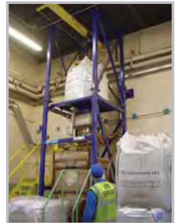
4. Bag loaded ready to discharge.
