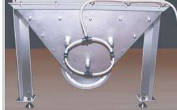
Inlet chute with aeration device.
