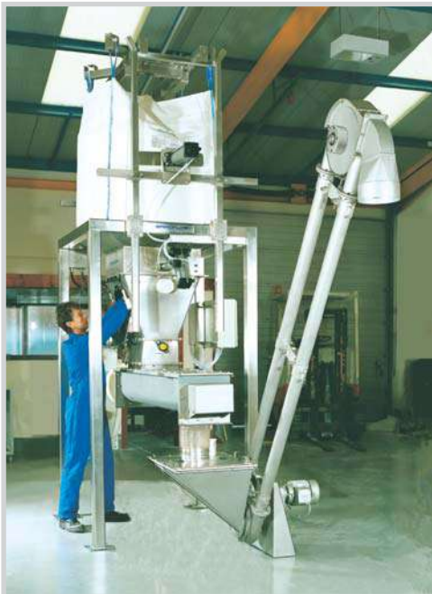
AMC designed for handling titanium dioxide. The aero mechanical conveyor is the only effective method of handling this type of product.
