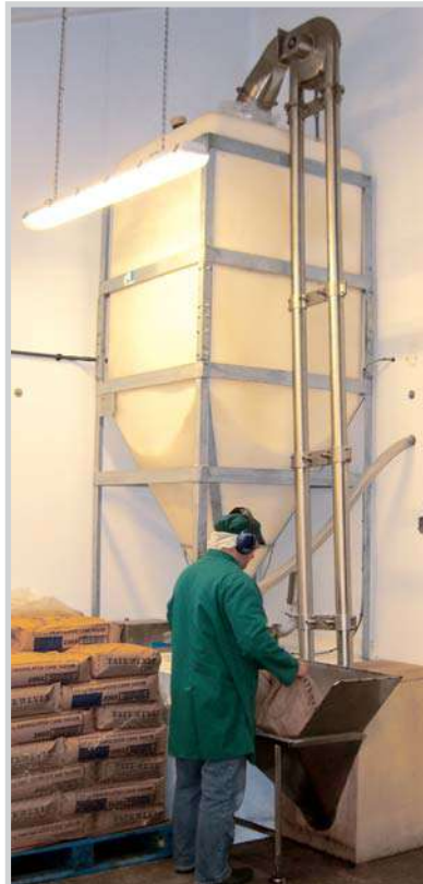
AMC elevating material from a transition hopper fed by two bulk bag dischargers via spiral conveyors.
