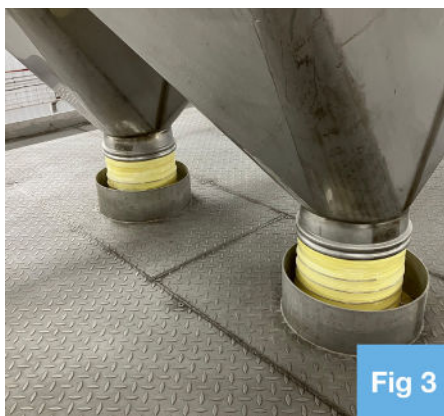
Adjustable filling with BFM® flexi connectors - Fig 3
