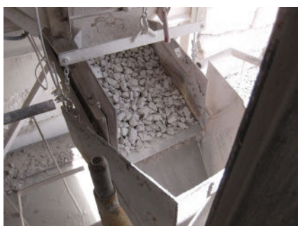
Bucket elevator inlet
