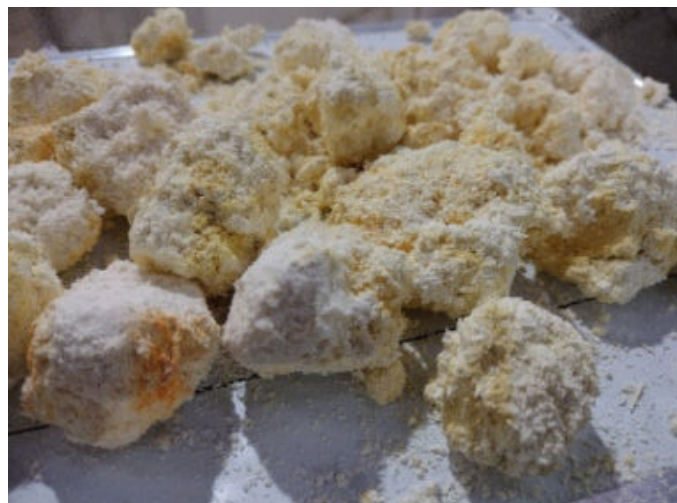
b) Caking due to mechanical load in the rapeseed waste
