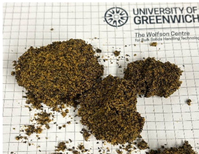
b) Caking due to mechanical load in the rapeseed waste
