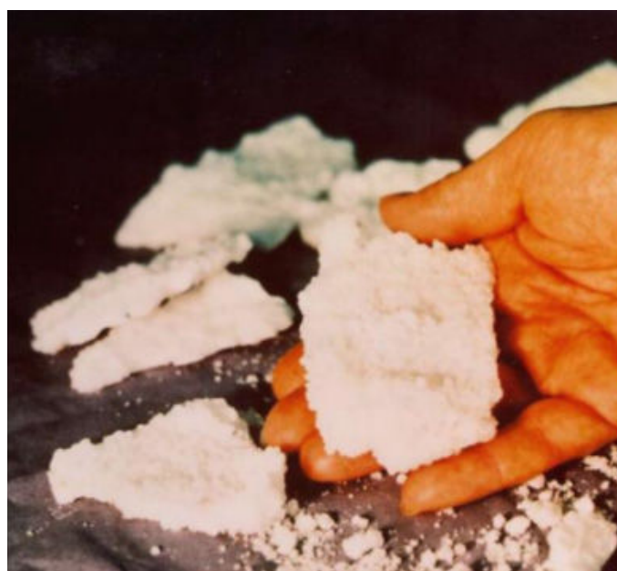
Figure 3: Caking phenomena in powder handling
