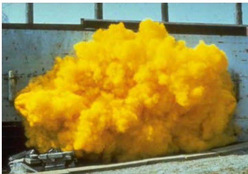
Figure 1: Optically dense dust cloud
