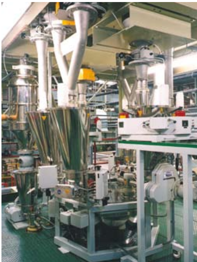
Modular volumetric and loss-in-weight feeders integrated with a gravimetric blending system and K-Tron PCS loaders in a plastics extrusion process
