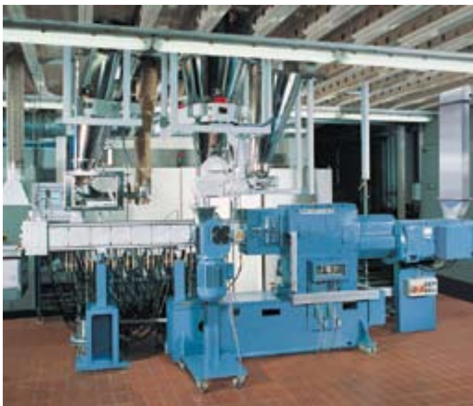
Loss-in-weight screw and vibratory feeders on a high performance extruder
