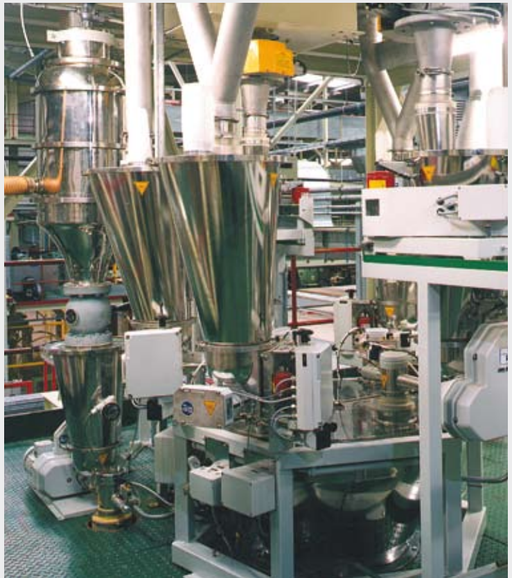
Modular volumetric and loss-in-weight feeders integrated with a gravimetric blending system and K-Tron receivers in a plastics extrusion process.
