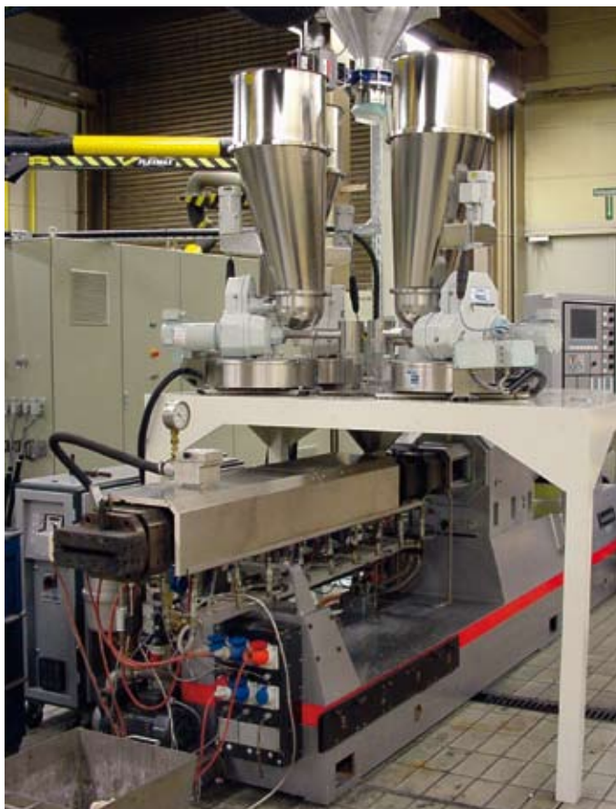
Modular loss-in-weight feeders arranged over an extruder
