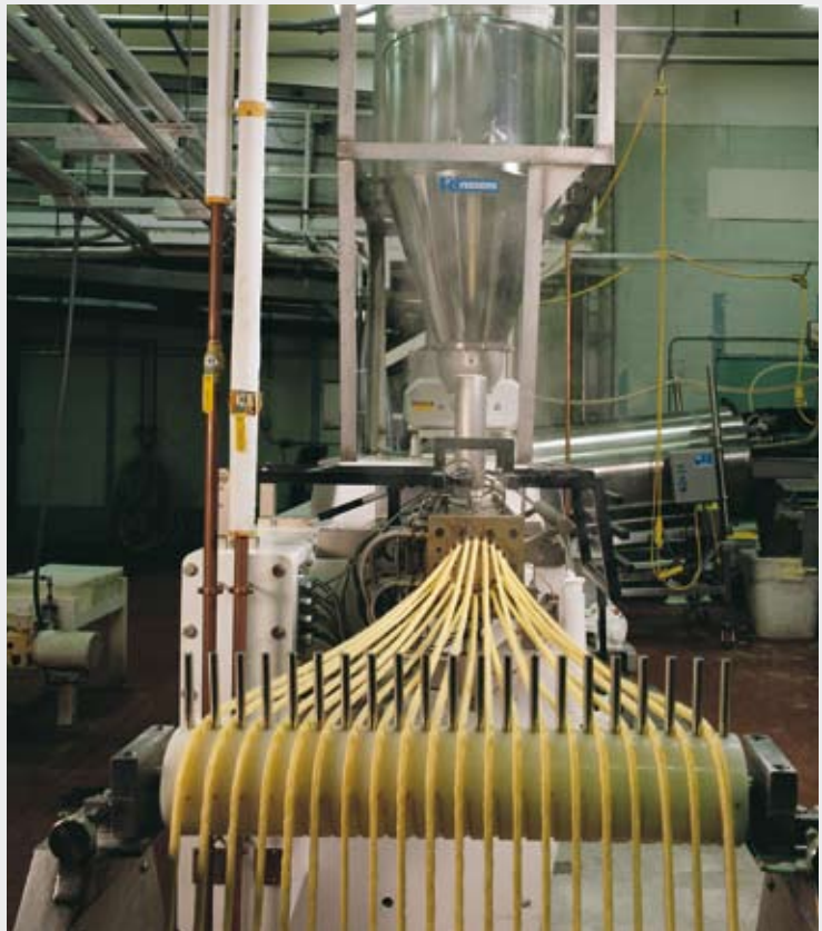
Twin screw modular feeder in snack food extrusion process.
