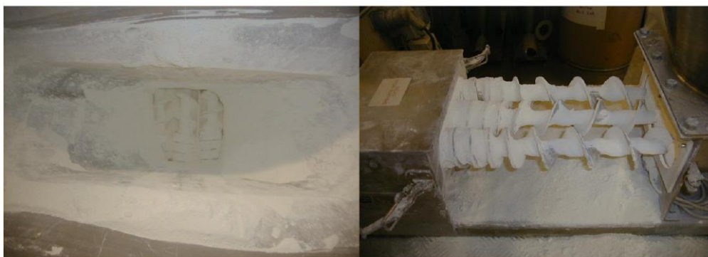
Figure 5: Titanium dioxide sticks to hopper walls and clogs screw feeder flights
