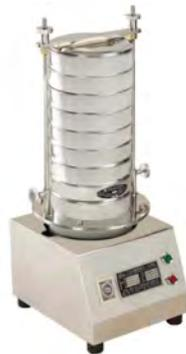
The quantity found on each mesh layer is then measured against the total to determine the percentage of each size range and to create a resulting graph. Below is a photo of a grain product showing the range of particle size in any given volume.
