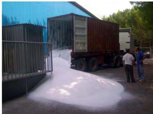
The decision on which material a liner should be manufactured from is influenced by the frictional force a given material has on the surface of the inside of the liner. Polyethylene film has a smoother surface property than woven polypropylene, even when coated or laminated, but this higher slip factor can also be detrimental. A fine balance is therefore
