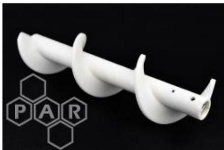
Augers and screw feeds (also known as flexible spirals or flexible screws) are more commonly used in the solids handling and processing industry for the compacting, dosing and bulk transfer of product such as flakes, granules and powders. They are typically manufactured from UHMW polyethylene, acetal or nylon, providing advantages over metal versions such as noise reduction, lighter weight, lower friction and improved product release properties.
