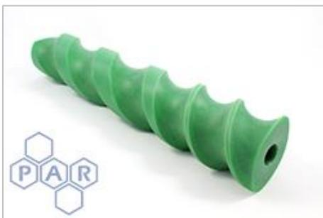
Timing screws and scrolls are complex engineering plastic components that are used to guide bottles, cans and containers through packaging, filling, capping and labelling lines within the brewing, beverage and food industries. They are typically manufactured from UHMW polyethylene or acetal and can be machined in various colours. They often integrate with plastic change pats which can also be manufactured by PAR.
