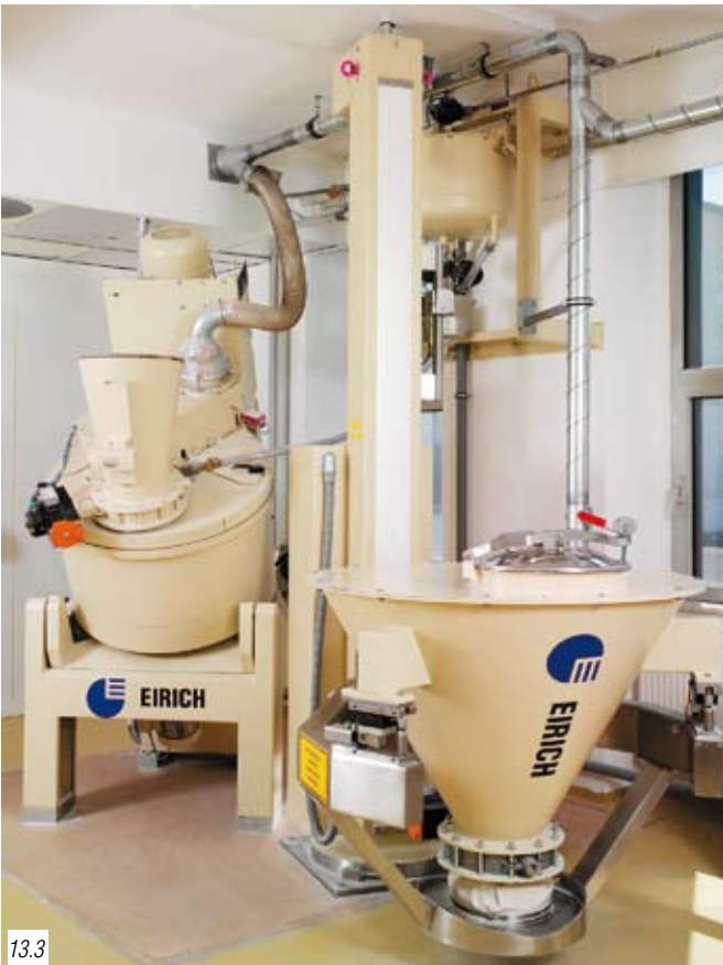
Fig. 13.1: Scale assembly Fig. 13.2: Additive storage and feeding Fig. 13.3: Mixer with infeed by elevator Fig. 13.4: Control room with CAQ system
