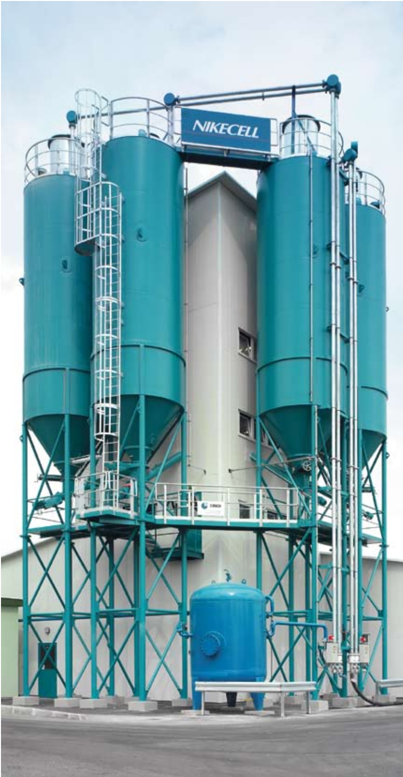
Fig. 12.1: Building and silos of a plant for adhesive mortar
