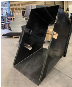
Ash hopper during fabrication as a direct replacement to an existing unit.
