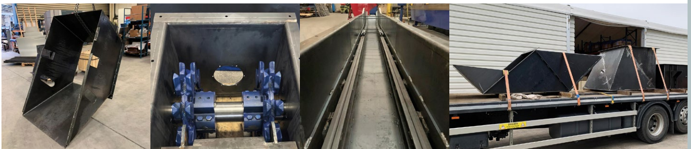
Ash hopper during fabrication as a direct replacement to an existing unit.
