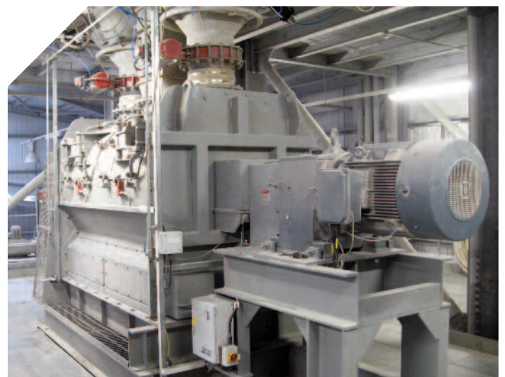
Highly energy efficient Delta Blade mixer reduces energy usage at F Ball Ltd
