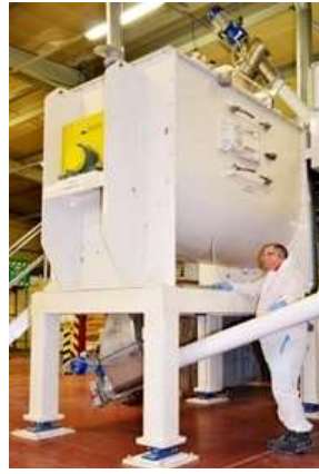
Figure 1 4000 litre John R Boone HHBM keeping the mix moving
