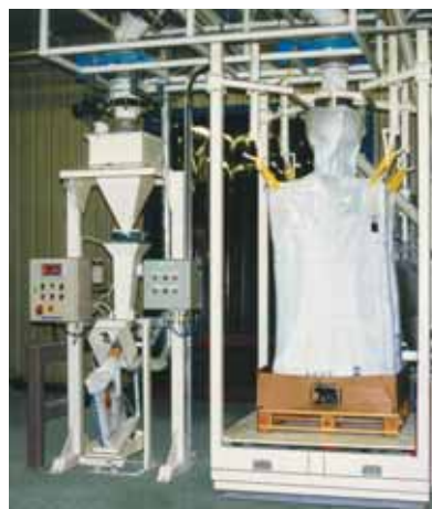
Filling system for bulk bags and sacks.
