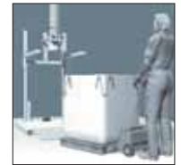
When filled, bag is removed by pallet truck.
